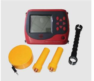
•TC600 rebar corrosion detector is desiged for assessing the corrosion of the reinforced concrete structure and components by half-cell potential method, the electrode goes through the surface of the concrete and the potential voltage difference is recorded, then the corrosion of rebar is assessed.
