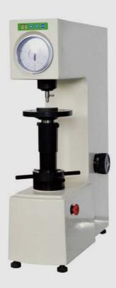
TIME6104 Double Rockwell hardness tester is a popularly-used hardness testing instrument to measure the Rockwell and superficial Rockwell hardness of the materials. It adopts the mechanism of automatic loading and unloading of the test force, the test force is regulated by the load-change hand wheel. It can select the dwell time and is very easy to use. Besides setting zero to dial, there is no man-made error. The instrument has high sensitivity and stability.
