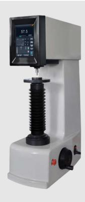
TIME6106 Automatic double Rockwell hardness tester with a good aesthetic aspect, complete functions, easy operation, intuitive display and good reliability, is a high-tech product combining the mechanic and electric features, which is suitable for the Rockwell and superficial Rockwell hardness test.
