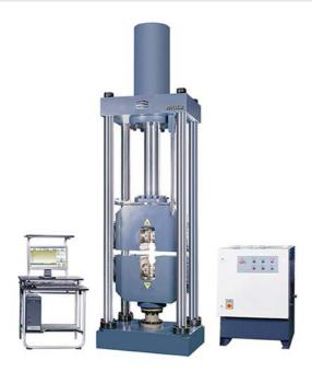
WAW- E Servo Hydraulic Tensile Testing Machine is mainly used for tensile test with high efficiency requirement. Equipped with relevant fixtures, this machine can also be used for compression, bending and shearing tests. Constant strain, Constant stress and constant displacement test are available. Strain velocity, stress velocity and displacement velocity conform to the requirement of GB, ASTM, DIN, ISO, JIS, BS etc. metal tensile testing standards.
