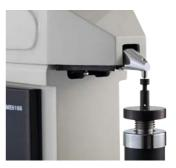
Surface hardness test of pin shaft
