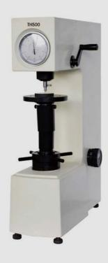
TH500 Rockwell hardness tester is a popularly used hardness testing instrument to measure the Rockwell hardness of the materials. No need for power supply, the speed of the test force loading is regulated by the buffer and the test force is regulated by the load-change hand wheel. It has easy operation and stable performance, therefore it is widely used.
