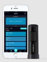
TCS-100 is an innovation color measuring tool with powerful configuration to make color measurement easier and more professional; It support Bluetooth to connect with Android and ISO devices, ColorMeter Pro will take you into a new world of color management; It can be widely used to measure color value, color difference value and find similar color from color cards for printing industry, paint industry, textile industry, etc.
