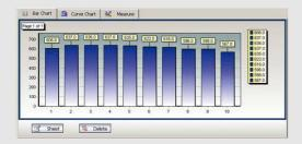
Dataview TH51X is special software for TH51X series Hardness Tester. The data stored in the Hardness Tester TH51X series can be transferred to the PC for further analysis with Dataview TH51X. It has online measurement mode and offline analysis mode, data analysis, graphics display and print output functions are all available.
