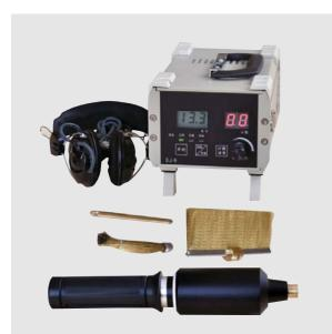
DJ series are designed for quick inspecting a wide range of non-conductive coatings and linings for pinholes, porosity and other faults by means of pulsed voltage in the non-destructive testing field. It is widely used in the petro-chemical, pipe mills, plastic fabrication and aerospace industries.
