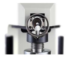
Ring/pipe inner wall hardness test
