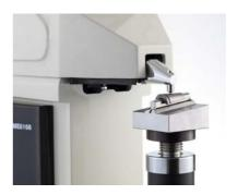
Hardness test of anchor clip
