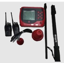
• TC300 is used for measuring the thickness of nonmetallic plate indirectly, especially for concrete slab. This gauge is to measure the concrete slab thickness mainly by using distribution characteristics of electromagnetic field and possesses function of thickness measurement, data analysis, data storage & output etc. it is a kind of intelligent thickness measuring instrument that is portable, convenient and accurate.
