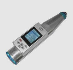
•HT225-V is a portable instrument to test the compressive strength of concrete structures or rock in non-destructive testing field. The rebound value can be converted into a reading on the digital display, and the estimated mean value, standard deviation and concrete strength can be shown.
